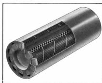
An air cleaner with a paper cartridge for effective filtration and damping of the high-frequency intake sound.
