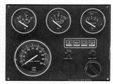
The instrument panel has clearly marked ISO symbols for temperature, oil pressure and charging. Double cover glass over instrument to prevent condensation. Key switch with starting and stopping functions and built-in starter motor protection.
