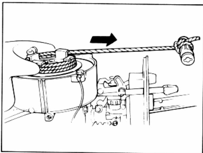
5. Tie a knot in one end of the emergency starter rope located in the tool kit. Tie the other end around the screwdriver handle in the tool kit.
