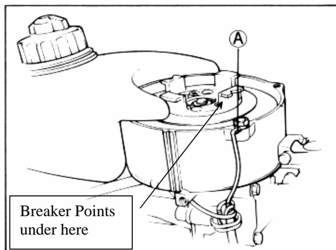
3. Bolt down the cable (A) with one of the bolts you just removed.
