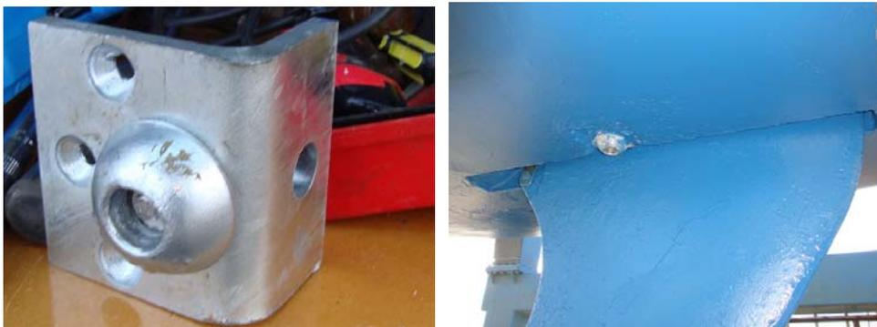
I painted the pivot holes on the angle brackets before inserting the new pin and greased the main nylon bearing to ensure that the pivoting would be in the correct place in future. I used plenty `Sikaflex marine sealant 291' to ensure a good seal around the bolts.
