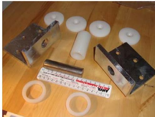
The job was reasonably straight forward but the new bracket holes didn't align correctly which was a bit of a pest to say the least! CHECK THE HOLE ALIGNMENT BEFORE APPLYING ANY MASTIC! The brackets were ordered from Beneteau and £50 a piece. They are 10mm galvanised mild steel (not Stainless). If I did this again I'd have the new brackets fabricated in stainless.
