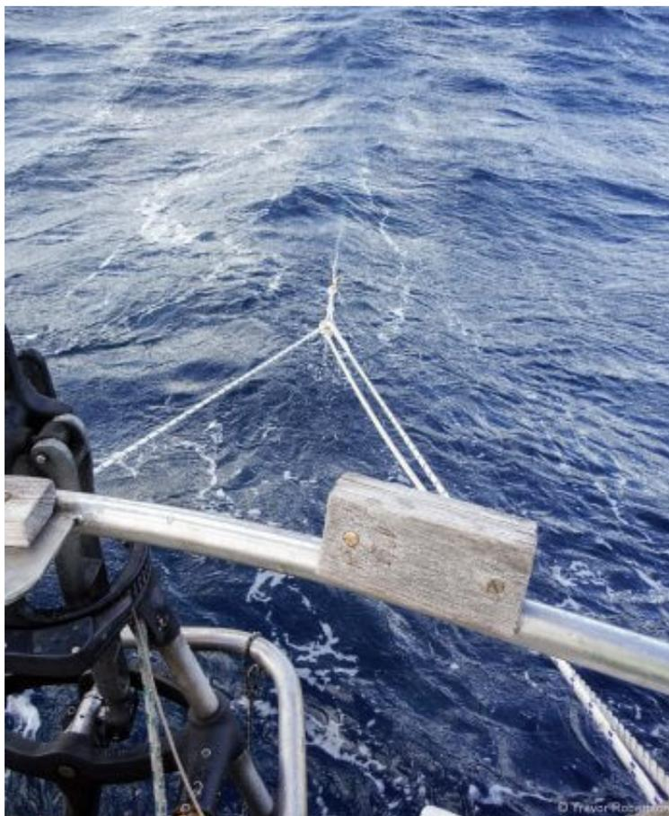
Before deploying the drogue I tied a stout rope to the junction of the bridle legs and the drogue leader. This third leg to the bridle is a lazy line that I kept under just enough tension to stop it fouling on anything without taking any strain. The line makes it easier to get the first few metres of the drogue in on retrieval, but its chief function is to allow me to steer across the wind by up to 30°.
