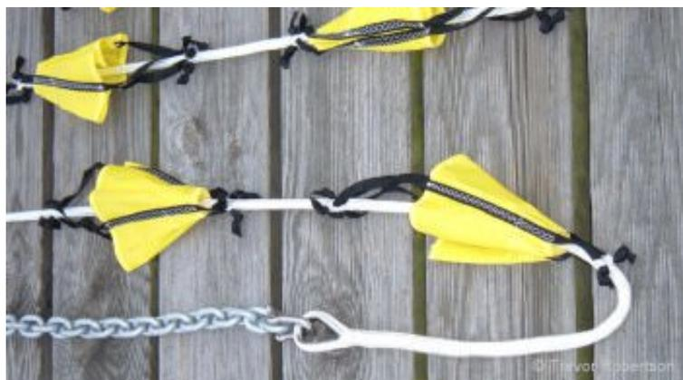
I used chain for the tail weight as it is easier to stow, deploy and retrieve than an anchor or a pig of lead
