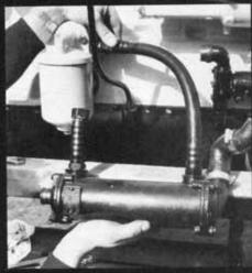
After the interrupter, the cooler. This small unit is connected to the water pump and to the interrupter. Oil passes through it one way, and water the other. The cooler can hang from its pipes or you could make up a supporting bracket that bolts to a couple of sump bolts.
