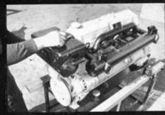
19. Two studs are now screwed into the bolt holes exposed when you removed the thermostat housing. The studs locate the fresh water heat exchanger and header tank. The thermostat we referred to earlier goes in under the header tank, and don't forget a new gasket. A blanking plug or a sender for a temperature gauge should be screwed into the thermostat bleed hole.
