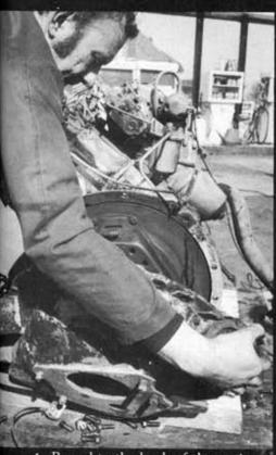
4. Round to the back of the engine now, and before starting to remove the bell housing make sure that the engine is blocked up on the sump, clear of the flanges and mounting feet. Unbolt the bell housing but keep all the bolts. The housing and clutch cylinder which is attached to it should join the scrap.
