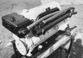
20. The end caps of the header tank can be turned by slackening the central bolt. The manifold end should have its pipe horizontal, the other side should point downwards. The pipes are now connected. The horizontal one has a pipe attached, running to the fitting on the far end of the exhaust manifold. The front end fitting on the manifold is connected to the point where the cooling water is injected into the exhaust stream. This prevents air
