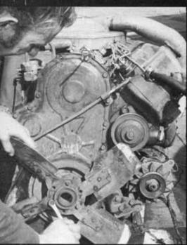
1. Block up the engine securely on the ground or on a platform so that it will be easy to work on and so that it will not fall on you when exerting pressure to loosen stubborn bolts. You are now ready to start the operation. The first step is to unbolt the fan from the front of the engine, a simple job requiring the removal of six bolts.
