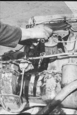
3. The air cleaner now comes off, but watch out for the oil inside. The fuel filter is usually bolted to the air cleaner bracket but don't disconnect the pipes, just remove the fastening bolts and let it hang on the pipes for the time being. The cleaner and piping are consigned to the scrap heap.
