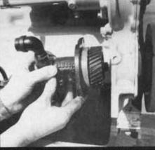
14. With your gleaming motor looking like new on its stand, start assembling the marine bits. First to go on is the water pump. This is a Jabsco gear-driven unit that fits into the space left where the air brake compressor came out. It bolts in with the old bolts.
