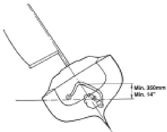
**⚠️ IMPORTANT!** Residual water must flow to silencer or overboard when the engine is shut off.
