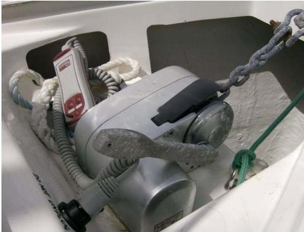
If you lose power to your windlass, start the engine and give it some revs, to make sure you have not just got a low battery voltage. Then make sure the windlass breaker with the anchor icon is in the 'on' position on the 12 volt panel. If there is still no power, check the location of the windlass fuse and make sure this has not tripped out. If you still have no power, you can operate the windlass manually.
