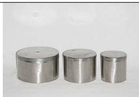
**Flange** - Made of stainless steel. Dimension: 70 mm – 90 mm – 114 mm
