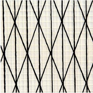
CSF's unique warp orientated polyester laminate is designed to be used for a variety of one design and small keelboat applications. The cloth is ideally suited for radial construction of sails for club and school fleets, our RDL cloth exhibits good durability as well as performance with Zero crimp warp yarns and overall stability.
