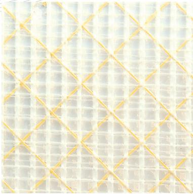
Our Radial Pentex Laminates (RPL) is a film on film laminate with Pentex warp fibres. Polyester is used in the weft giving a combination of a virtually zero crimp Pentex warp with a softer Polyester fill to prolong competitive use. A 45° black Polyester scrim reduces the film loading and stabilises the bias.
