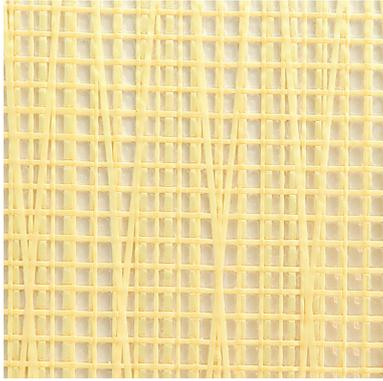
Our Aramid Racing Laminate (RAL) is ideal for racing applications up to 55 feet.
