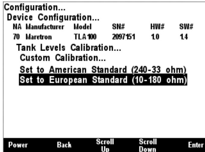
Figure 195 – European Standard Sender Calibration
