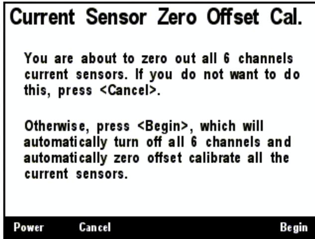
**Figure 54 – DCR100 Current Sensor Zero Offset Calibration Screen**
