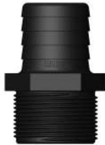
TruDesign Tails are moulded from a glass reinforced nylon composite. High strength, high-modulus glass fibers impregnated into the nylon provides dramatic strength, stiffness, toughness, and dimensional stability. TruDesign Tails eliminate the corrosion and electrical bonding problems associated with metallic fittings. The Tails are designed for twin hose clamps, and do not crush under high load conditions.
