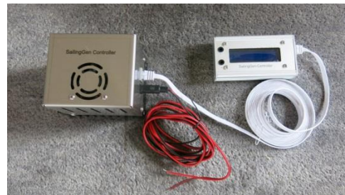
SailingGen-Controller, consisting of the Controller-Box and the LCD-Display
