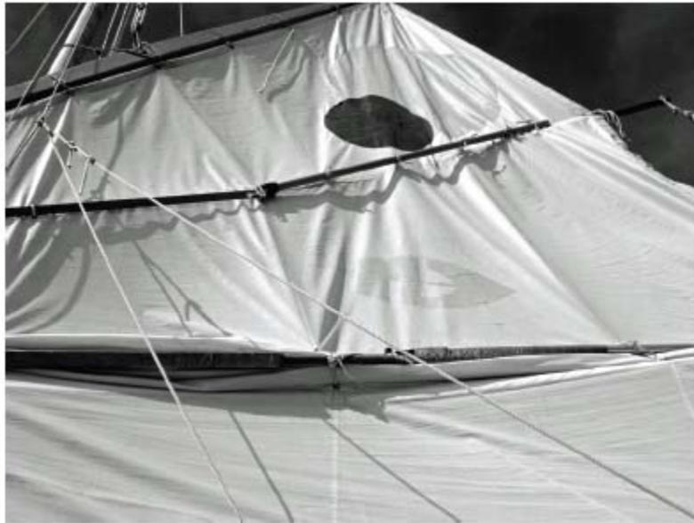
*Mingming's jury rig, mainly boat hooks and gaffer tape. We sailed well over two thousand miles under these patched up battens.*
