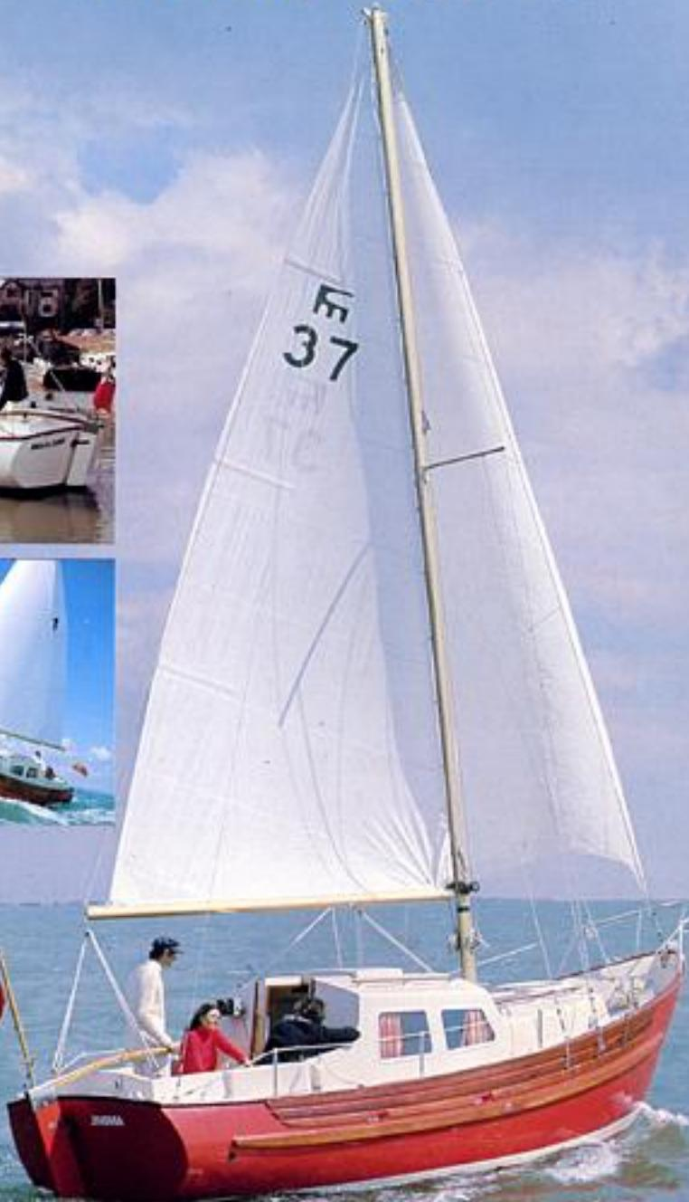
The Freeward version of the 25' offers for the more orthodox taste of the cruising yachtsman who wants a rugged seaworthy sailing sloop with an open cockpit. Using the Fisher class hull, she has a different deck mould and accommodation layout which is exceptionally comfortable for a couple or family. Her flexibility of purpose and heavy duty construction are equally suited to the sailing beginner pottering around coastal waters, or transocean voyages of which several have been conducted.
