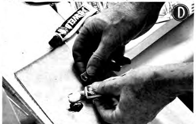
D: We're recommending J-B Weld to secure the flange to the hull. It's not that easy to buy (but Jaycar stores do stock it – Cat NA1518) and it's not real cheap – but it sticks like the proverbial.
