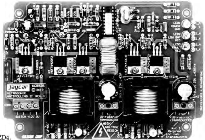
two TP GND points. Following these, mount the diodes, which must be orientated as shown in Fig.5. Note that there are several different diode types: 1N5819s for D1-D4 and D10; UF4007 for D5 and D6; 1N4004 for D7; BAT46 for D8 and D9; and 5.1V zener diodes for ZD1-ZD4.
