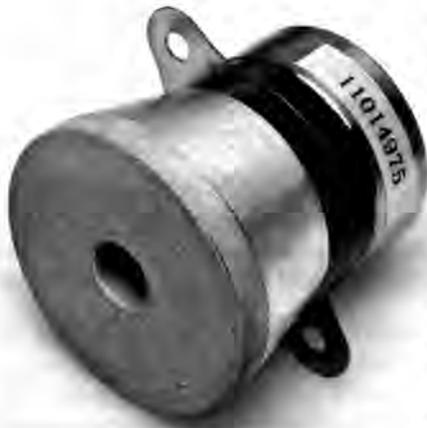
(Left): here's the "business end" of the system, the Ultrasonic Transducer, which sets up the vibration pattern in the boat hull which marine vegetation doesn't particularly enjoy! Because these operate at high voltage (~700-800V peak-to-peak) they must be fully enclosed ("potted") in a suitable enclosure, as shown above. (The Jaycar kit will have potted transducers).
