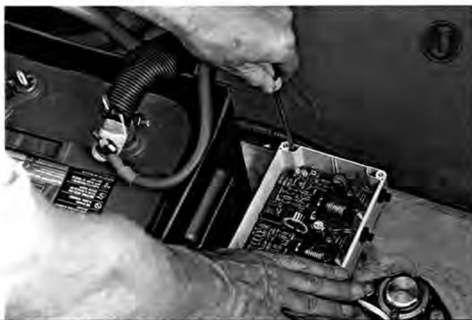
**J:** Use good quality marine stainless steel screws for securing the case to its mounting position. A power screwdriver is a good idea here: we didn't have the right bit and screwing into the fibreglass was really tough going.
