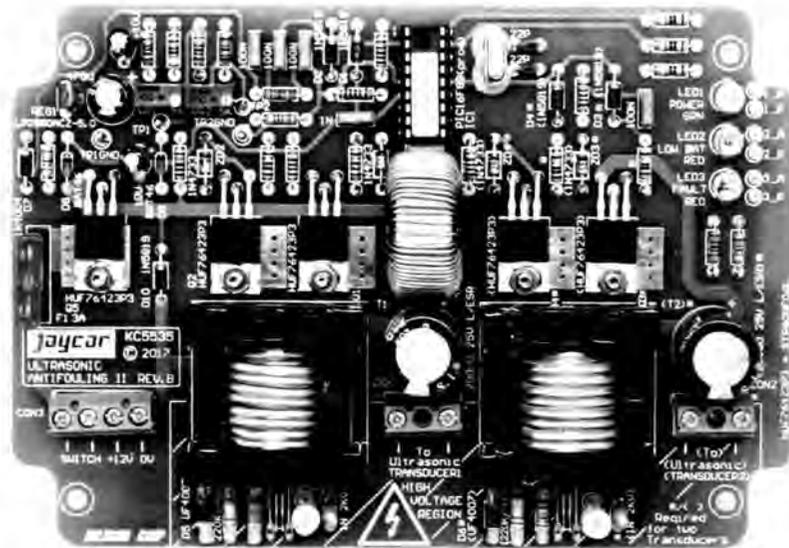
Mosfets Q3 and Q4 in the same manner. The microcontroller runs at 20MHz (using crystal X1) and this allows it to provide the small ultrasonic frequency shifts required.
