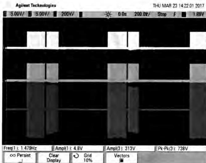
Fig.3: taken at a low sweep speed of 200ms/div, this scope grab shows that the transducer is driven in two frequency blocks, as described in the text.
