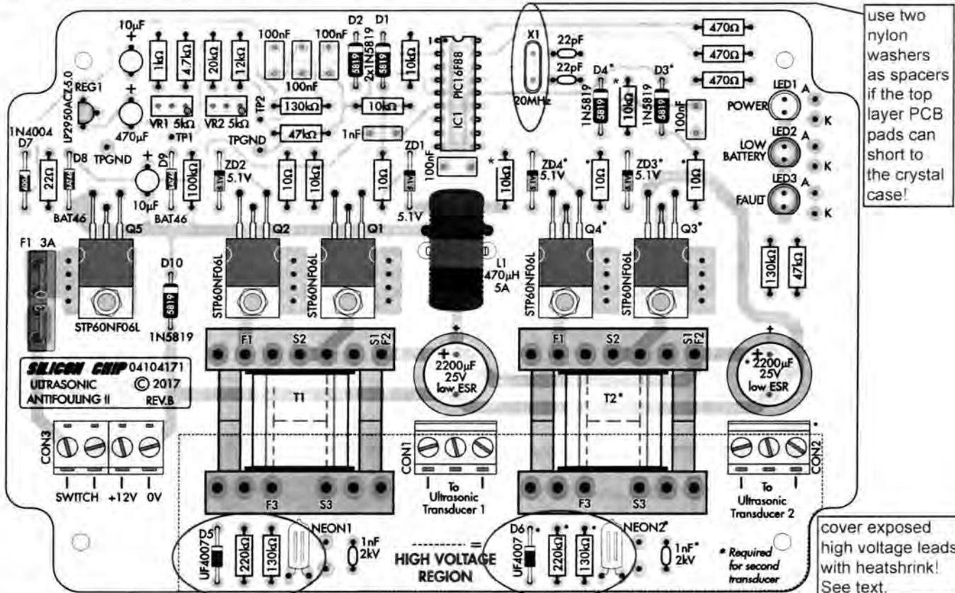
Fig.5: component overlay for the two transducer version of the Ultrasonic Anti-Fouling Unit, MkII. To build the single transducer version, simply leave out all components in the light yellow section of the PCB – Q3, Q4, ZD3, ZD4, D3, D4, D6, NEON2, T2, CON2 and associated resistors/capacitors. Note the area of the PCB with a dashed red border/light pink background has high voltages on both the tracks and component leads when operating.
