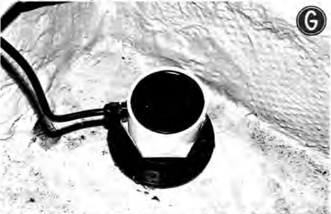
G: Once set (24 hours +), the transducer assembly is screwed into position with a good big dollop of Fix-A-Tap lubricant on the face. But before doing so, wind it anti-clockwise a number of turns.
