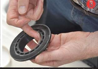
B: It's important that glue doesn't get into the thread, where it would clog it up. Smear a good coating of Vaseline right around the threads – make sure it doesn't get on the bottom of the flange.
