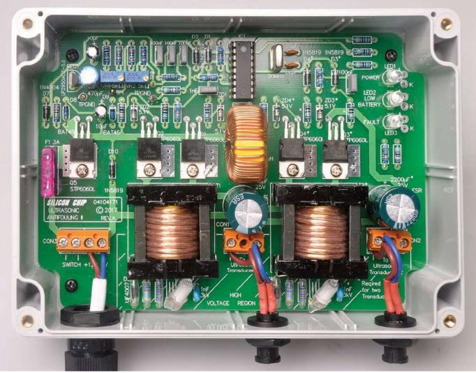
Here's what the PCB looks like mounted inside the waterproof polycarbonate box with external connections made . . .
