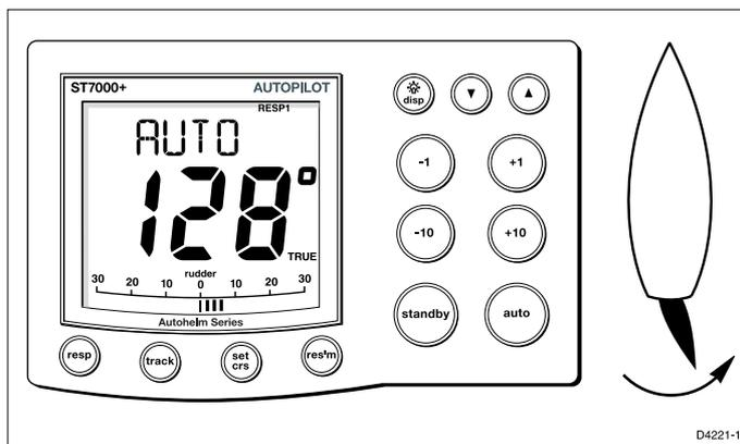
4. If the helm produces a turn to port, reverse the motor connections at the course computer.
