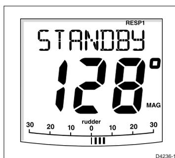
This shows that the control head is active. If the above events do not occur, check the fuse/circuit breaker.
