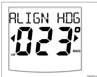
8. Use the **+1**, **-1**, **+10** and **-10** keys, to adjust the displayed heading, until it agrees with the ship's steering compass or a known transit bearing.
