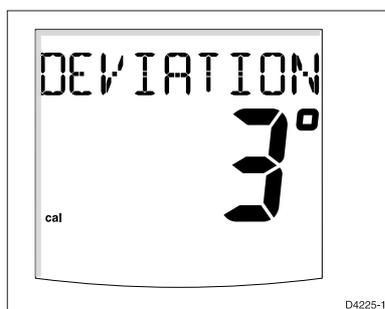
This shows the maximum deviation detected, and indicates that compass correction has been completed successfully.
