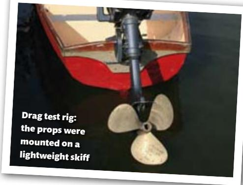
Drag test rig: the props were mounted on a lightweight skiff
