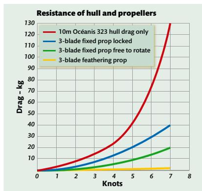
At 5 knots, a fixed three-blade prop with its shaft locked creates almost half as much drag as the entire hull. The drag can be halved by allowing the prop to spin, but the gearbox may suffer.
