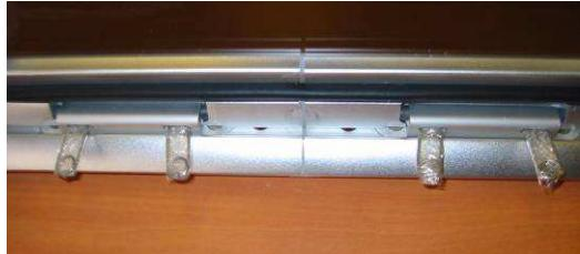
Remove the spring pins one after the other and slightly lift up the lid in order to engage the hinges completely.
